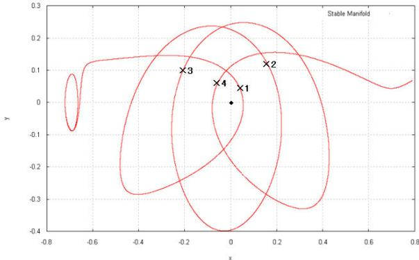
**Fig. 5: First Four Periapsis Passage Points of one example trajectory of the stable manifold propagated backward for  $J = -2.15$ .**
