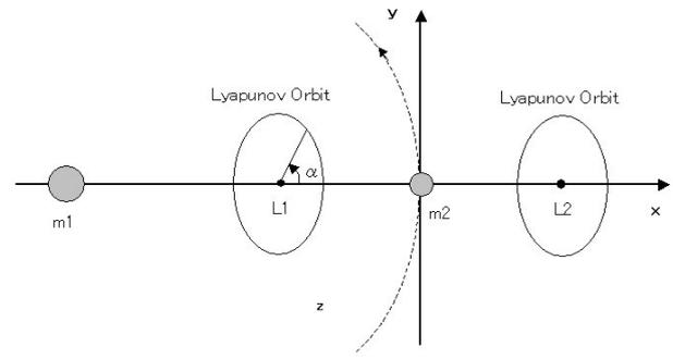
**Figure 2: Geometry of the planar Restricted Hill Three-Body Model**
