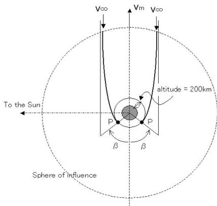
Fig. 9: Periapsis Location (angle  $\beta$ ) after Interplanetary Space for Hohmann Transfer.
