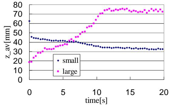
Fig.8. The average height of each size particles,  $z_{av}$ , as a function of time ( $A=35[\text{mm}]$ ,  $T=0.33[\text{s}]$  and  $R=3.0$ ).
