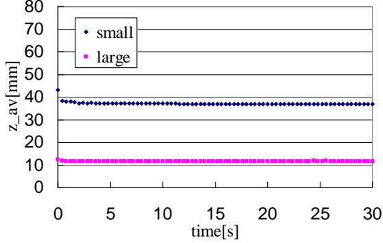
Fig.7. The average height of each size particles,  $z_{av}$ , as a function of time ( $A=35[\text{mm}]$ ,  $T=0.40[\text{s}]$  and  $R=2.0$ ).  $A(2/T)^2=8636[\text{mm}/\text{s}^2]$ .
