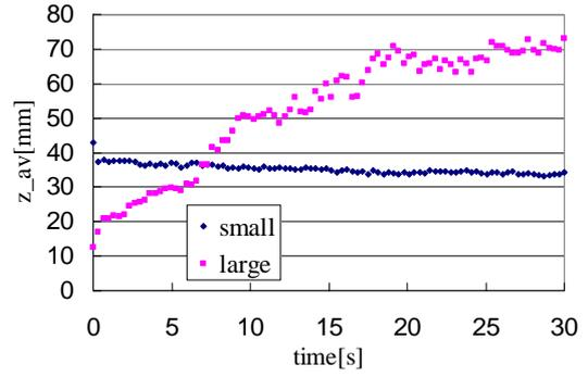
Fig.4. The average height of each size particles,  $z_{\text{av}}$ , as a function of time ( $A=35[\text{mm}]$ ,  $T=0.33[\text{s}]$  and  $R=2.0$ ).  $A(2/T)^2=12688[\text{mm/s}^2]$ .
