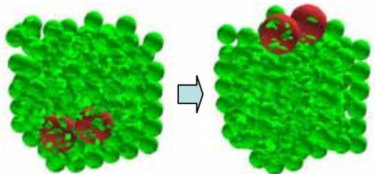
Fig.6. Images of the initial position and the position after shaking ( $A=50[\text{mm}]$ ,  $T=0.33[\text{s}]$  and  $R=2.0$ ), which show the Brazil nuts effect.
