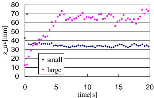
Fig.3. The average height of each size particles,  $z_{\text{av}}$ , as a function of time ( $A=50[\text{mm}]$ ,  $T=0.33[\text{s}]$  and  $R=2.0$ ). Maximum wall acceleration,  $A(2/T)^2=18126[\text{mm/s}^2]$ .
