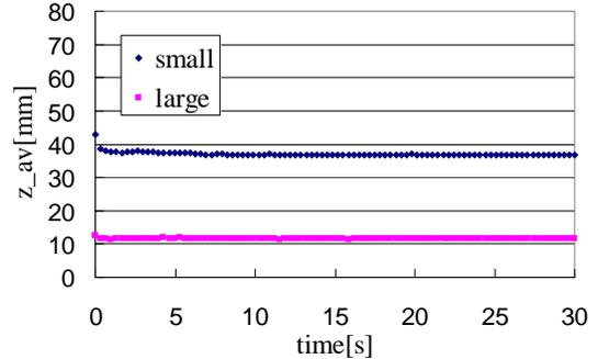
Fig.5. The average height of each size particles,  $z_{\text{av}}$ , as a function of time ( $A=25[\text{mm}]$ ,  $T=0.33[\text{s}]$  and  $R=2.0$ ).  $A(2/T)^2=9062[\text{mm/s}^2]$ .
