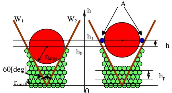
Fig.9. Concept of arch effect. The two-dimensional model of arch effect for calculating  $R_s$ . The left diagram is the initial stable condition by arch effect and the right one is the next condition where arch effect takes place.
