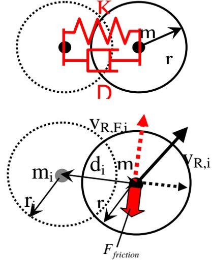
Fig.2. Schematic diagram of mass-spring-damper (MSD) model considering friction.
