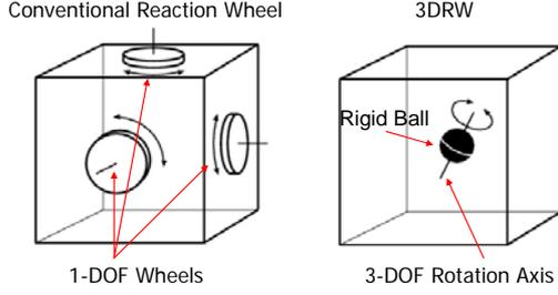
Fig. 1: Conventional reaction wheel and 3DRW
