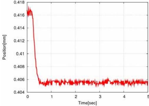
Fig.8: Experiment result of PID control
