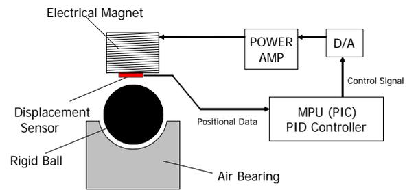
Fig.6: Diagram of the position control system
