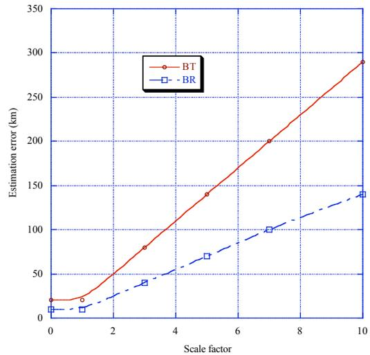
Fig. 5 Sensitivity of the estimation error to perturbation of random nongravitational accelerations (X-band two-way Doppler plus ranging)
