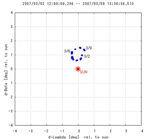
Figure 7 +Z axis history without thrust (Sun Tracking)
