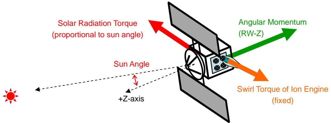
Figure 5 Solar Radiation Torque and Swirl Torque of Ion Engine
