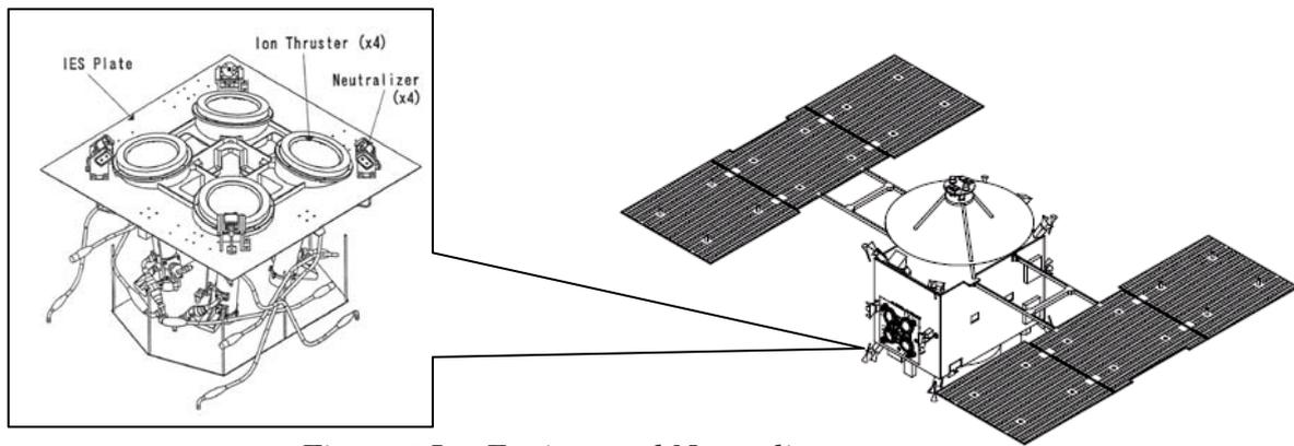
Figure 1 Ion Engines and Neutralizer
