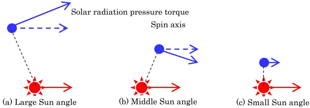
Figure 3 Relation of Sun direction and Spin axis.
