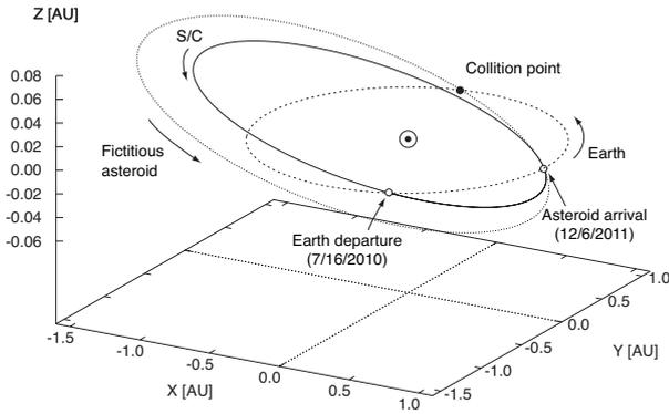
Figure 6. Optimal trajectory for nominal  $\Delta V$  case
