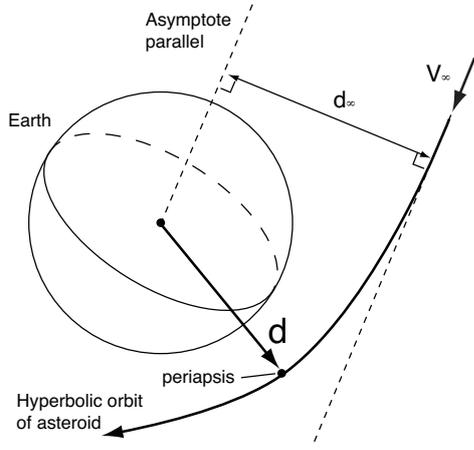
Figure 2. Hyperbolic trajectories of the asteroid in avoiding the collision to the Earth
