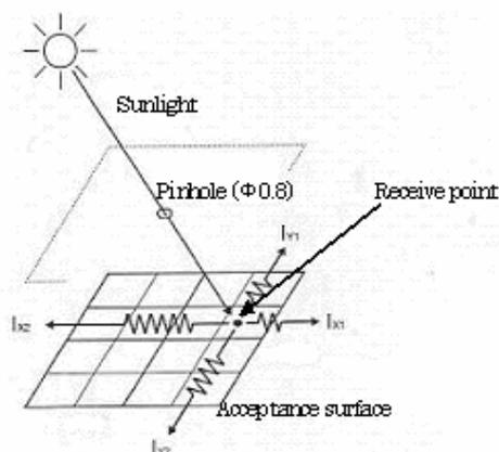
Fig. 3 Principle of Sensing the Sun's Light in PSD
