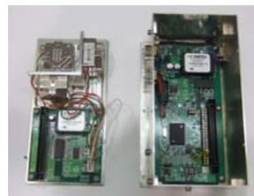
Fig. 6 Gyro Rate Sensor Unit
