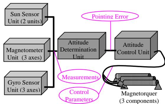
Fig. 2 Data Flow in ADCS
