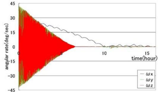
Fig. 12 Angular Rates under B-dot Control
