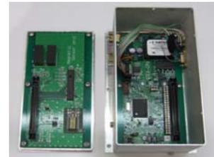
Fig. 5 Magnetometer Unit
