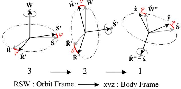
Fig. 9 Transformation from Orbit Frame to Body Frame
