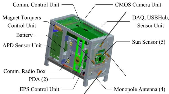
Fig. 6 Cute-1.7 + APD#2 Components Layout
