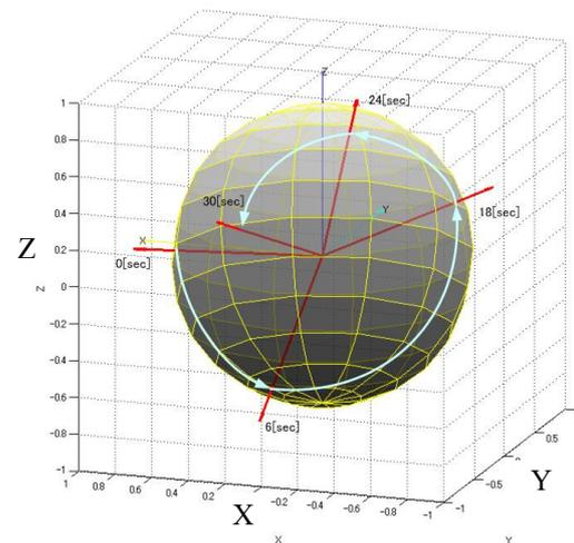
Fig. 5 Direction of the sun in body fixed coordinate system
