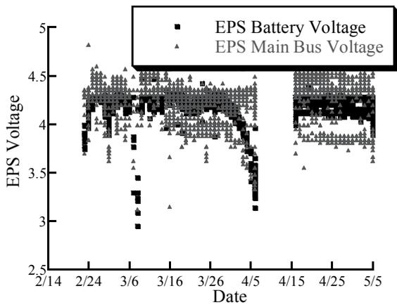
Fig.2 Flight Data of Battery and Main Bus Voltages
