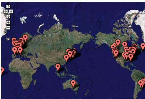
Fig.3 Reception reports from the world powered by google earth. Plots are the points where radio amateurs received the signal from Cute-1.7 + APD#1.
