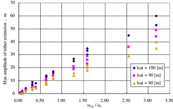
Figure 10 Dependency of  $A_{max}$  on  $\omega_{sc}/\omega_t$
