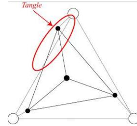
Figure 9 Unacceptable Configuration
