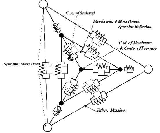
Figure 3 Numerical Simulation Model (Mass-Spring-Damper)
