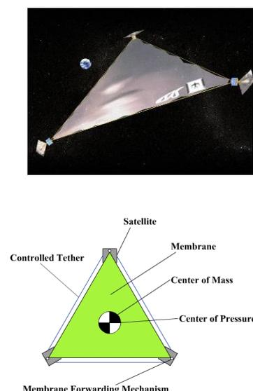
Figure 1 Tether-Controlled Spinning Solar Sail
