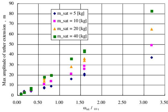
Figure 11 Dependency of  $A_{max}$  on  $\omega_{sc}/\omega_t$
