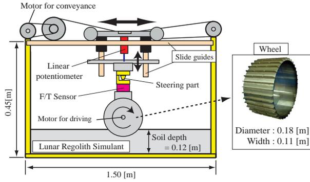
Fig. 3: Schematic view of the single wheel test bed
