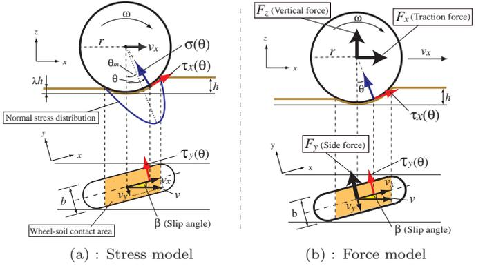
Fig. 2: Wheel-soil contact model
