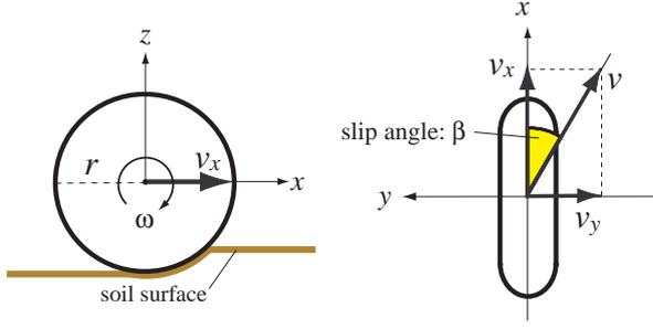
Fig. 1: Wheel coordinate system
