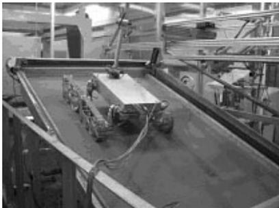
Fig.5 Testing configuration of hill climbing performance
