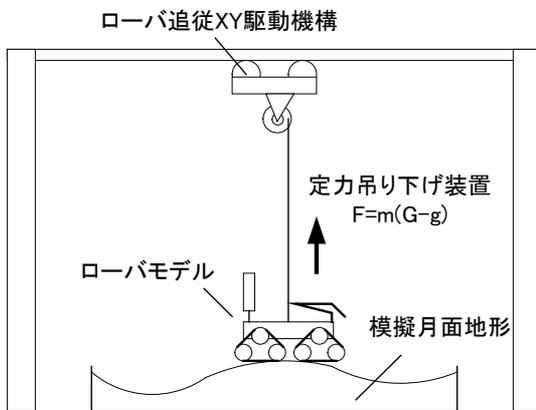
Fig.4 Gravity compensated rover testing configuration
