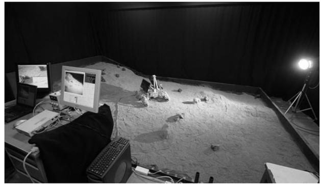
Fig.9 Lunar/Mars rover testing facility
