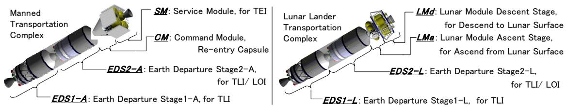
Figure 3 module description for 6-launch scheme
