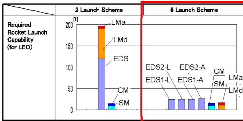
Figure 4 Comparison of 2-launch scheme and 6-launch scheme
