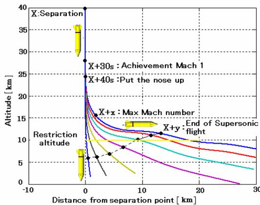
Fig.4 Flight path of each attack angle
