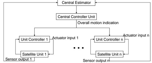
Fig. 1 Hybrid architecture for control of overall space structure
