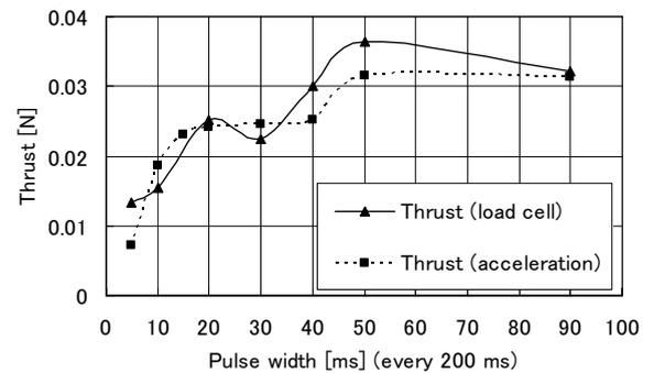
Fig. 4 Thruster property in relation to pulse width
