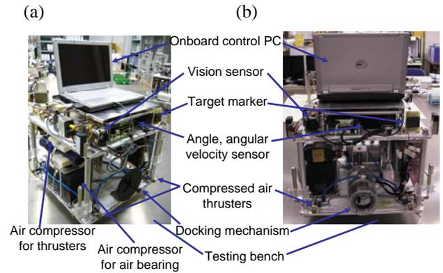
Fig. 3 Small satellite models: (a) chaser satellite and (b) target satellite
