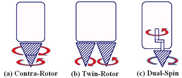
Fig.8 Schematic of N-RDM systems
