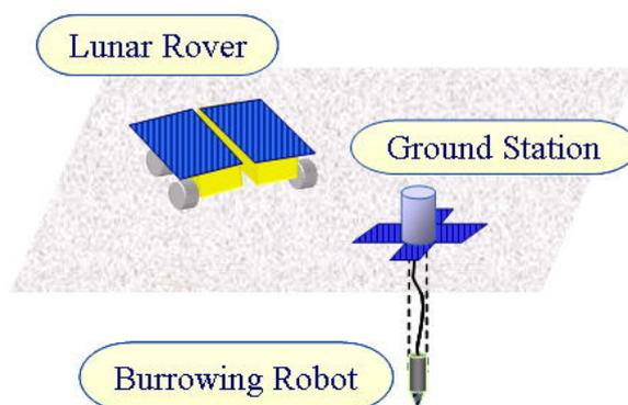
Fig. 1 Schematic of lunar subsurface exploration
