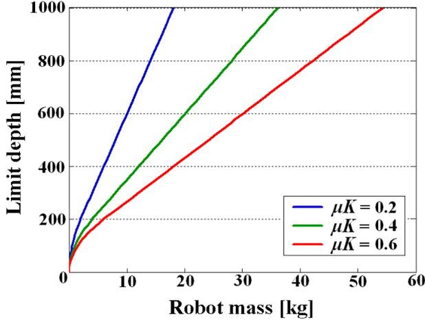
Fig. 5 Advancing limit depth by its weight
