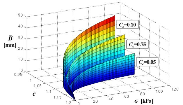
Fig. 7 Compression limit by Mohr-Coulomb's failure criterion with  $C_c$
