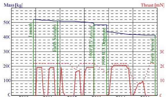
Figure 3 Mass and Thrust Profile of Nominal Mission Sequence
