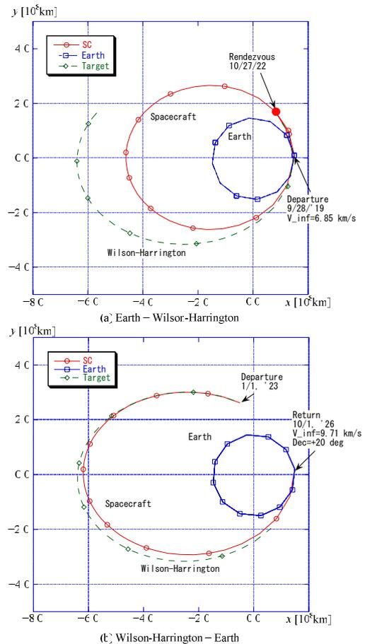
Figure A1 Trajectory Profile of Wilson-Harrington Exploration Mission (Rotational Coordinate System)
