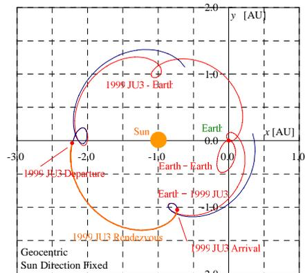
Figure 7 Trajectory Profile of Mission Sequence
