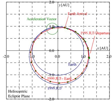
Figure 6 Trajectory Profile of Mission Sequence
