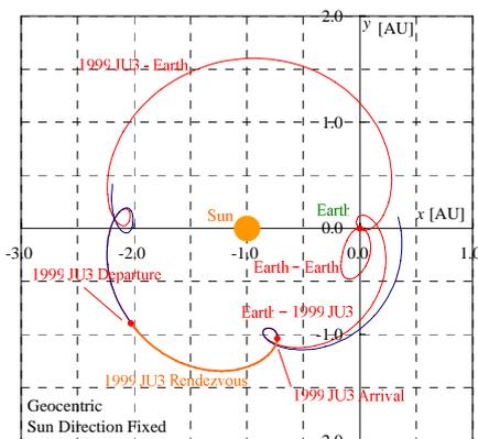
Figure 4 Trajectory Profile of Nominal Mission Sequence (Rotational Coordinate System)
