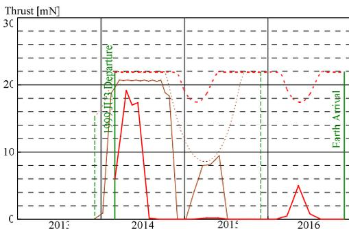
Figure 5 Thrust Profile of Mission Sequence
