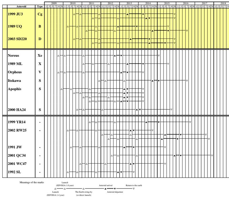
Figure 1 Near Earth Asteroid Sample Return Mission Sequences in Early 2010s
