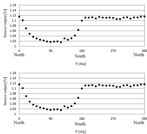
Fig. 4. Experimental results (thermopile sensor, night)
