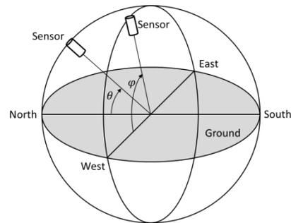
Fig. 2. Sensor direction
