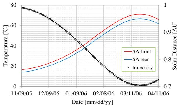
Fig. 5 Predicted VEX Solar Array Temperatures and Solar Distance
