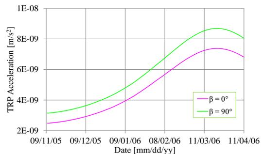
Fig. 9 Predicted TRP Acceleration during Cruise Phase
