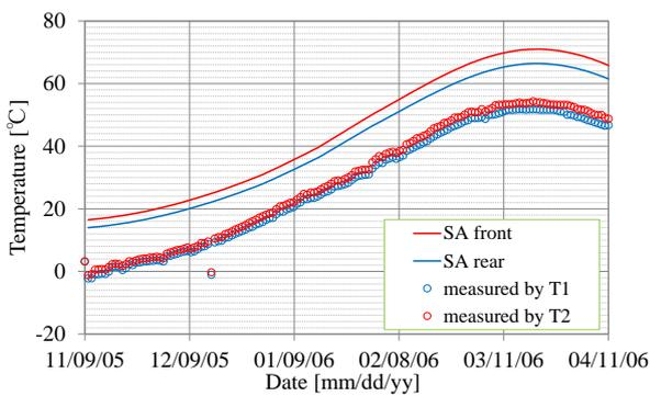
Fig. 6 Predicted vs Measured Array Surface Temperatures
