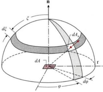
Fig. 1 Emission into a Hemisphere of Radius  $r$
