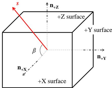
Fig. 3 Sun Vector Relative to Body Frame and Surface Normal Vectors
