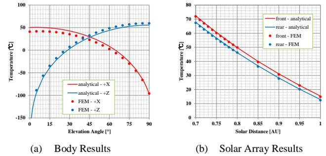
Fig. 4 VEX External Surface Temperatures of Body and Solar Array
