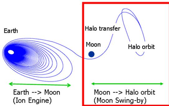
Fig. 2: Trajectory Design in DESTINY Mission.
