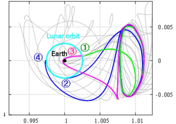
Fig.7: Transfer trajectories from the moon to the Halo orbit
