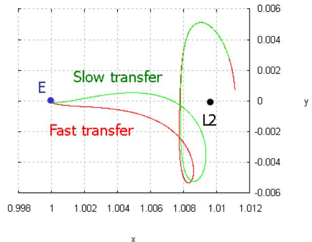
Fig. 1: Transfer Trajectory to the Halo Orbit Using the Stable Manifold [4]
