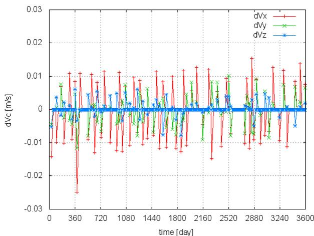
Fig. 6-2-1. Direction of Corrective Maneuver (L2-centered rotational coordinate system)
