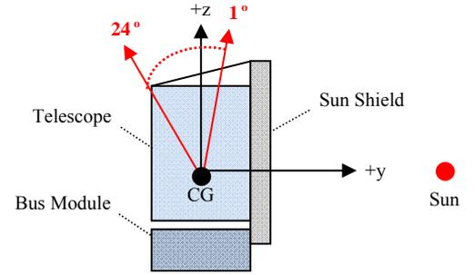
Fig. 4-1-1. Attitude Constraint of SPICA
