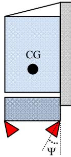
Fig. 4-2-1. Definition of the Cant Angle
