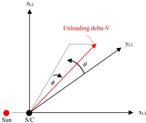
Fig. 4-2-2. Definition of the Unloading delta-V
