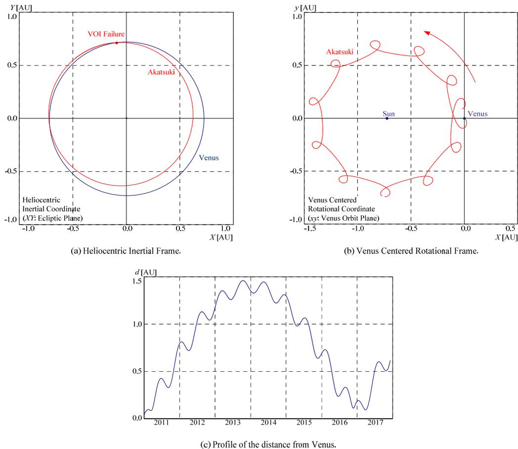
Fig. 1. Orbit of AKATSUKI after the Venus Orbit Injection Failure.
