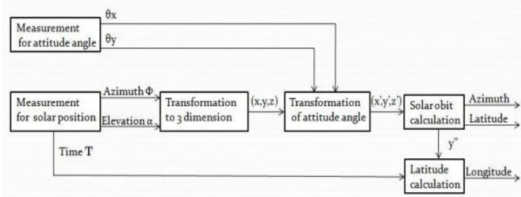
Fig.8 The block diagram of Mars positioning system
