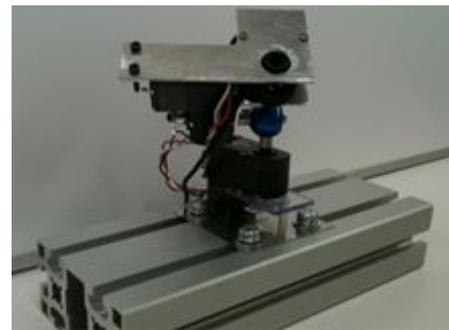
Fig.9 The solar tracking device
