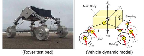
Fig. 4 : Vehicle dynamic model as an articulated multibody system.
