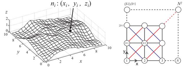
Fig. 1 : Terrain map represented by DEM. Right figure shows the node connectivity between the adjacent nodes.  $N$  is the number of nodes per length of the terrain map.
