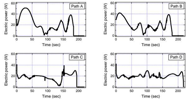
Fig. 8 : Time histories of the electric power used by the rover actuators.
