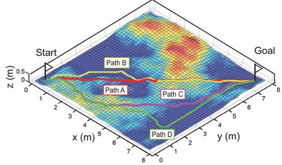
Fig. 5 : Terrain elevation map and typical candidate paths generated.
