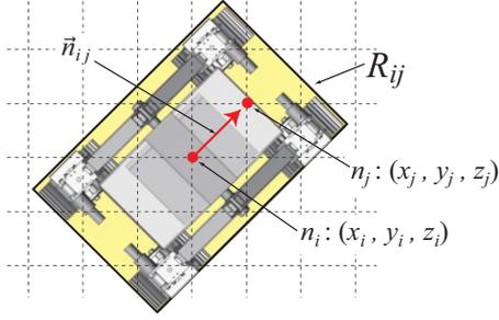
Fig. 2 : Projection region (yellow-colored area) of the rover on terrain map.
