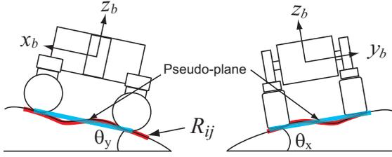
Fig. 3 : Terrain inclination angles. The red curvature depicts the projection region  $R_{ij}$  and the blue line depicts the pseudo-plane composed of wheel contact points.
