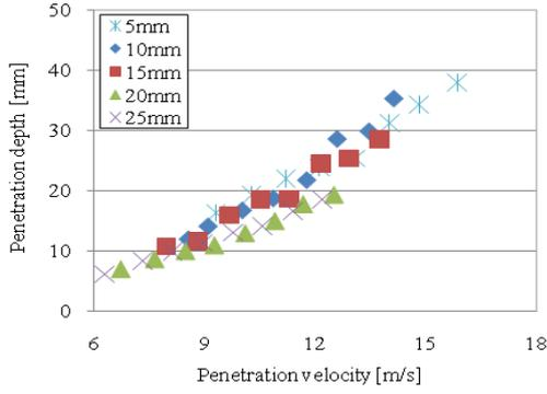
Fig. 8. Result of relation between penetration depth and penetration velocity (light concrete)
