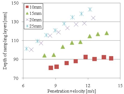
Fig. 6. Result of relation between depth of the sampling layers and penetration velocity
