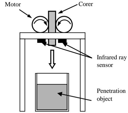
Fig.3. Schematic view of experimental device
