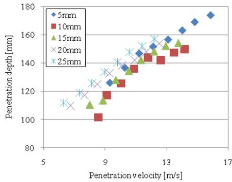
Fig. 5. Result of relation between penetration depth and penetration velocity (sand)
