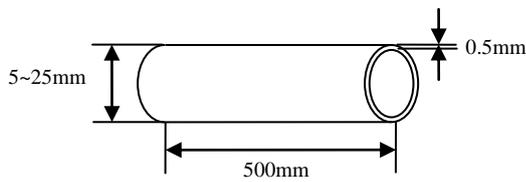
Fig. 2. Schematic View of Corer
