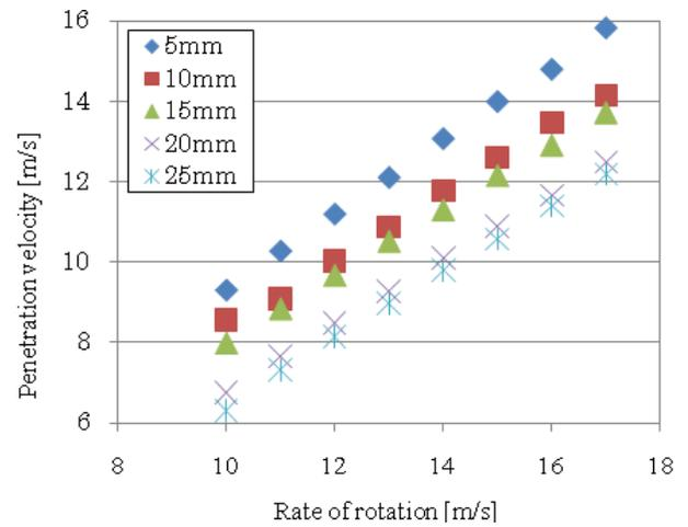
Fig. 4. Result of relation between penetration velocity and rate of rotation
