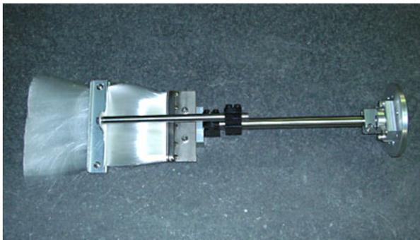
Figure 3 Prototype of brush-contactor
