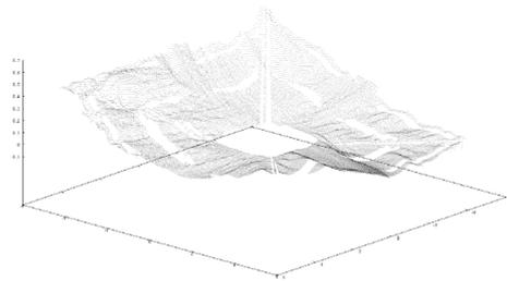
**Figure 12. Preliminary result of sail shape estimation from a camera image.**
