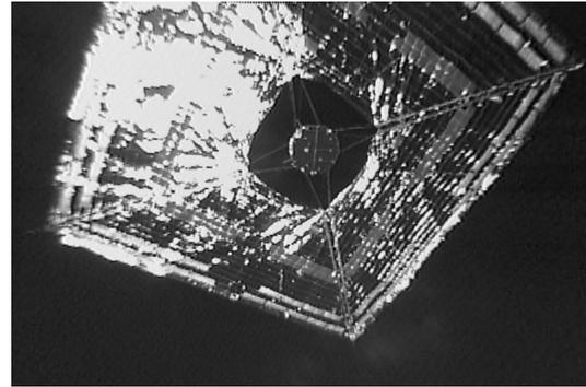
**Figure 11. An example of obtained image of the deployed sail. RCD is attached on the edge of the sail. This image was obtained by a small camera-carrying probe deployed from the**
