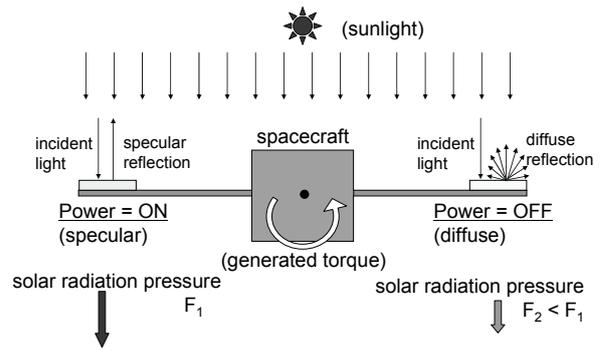
**Figure 3. Concept of proposed attitude control system using only solar radiation pressure.**
