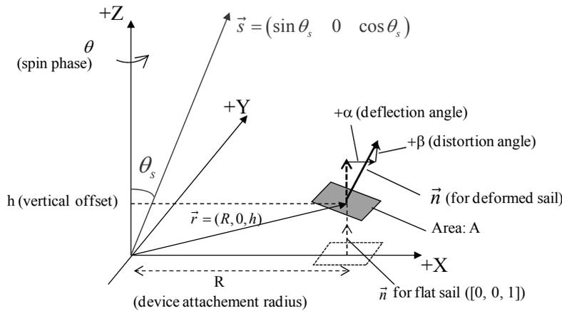
Figure 7. Definition of coordinate system and sail deformation.
