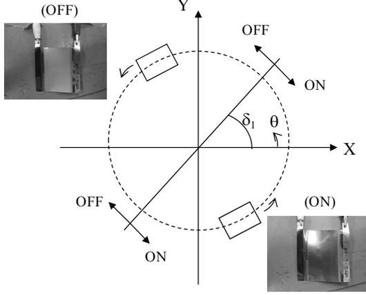
**Figure 8. Definition of switching control scheme and switching phase  $\delta_1$ .**
