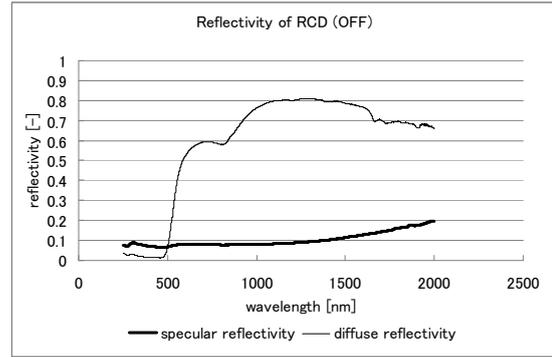
**Figure 5. Reflectivity of RCD when it is OFF.**
