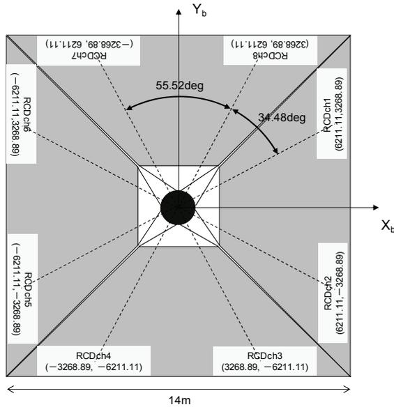
**Figure 4. Arrangement of eight blocks of RCDs on IKAROS' sail. The value in brackets indicate the coordinate of each blocks in the body-fixed coordinate system.**
