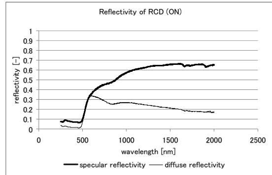
**Figure 6. Reflectivity of RCD when it is ON.**
