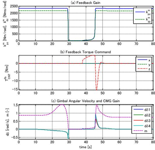
Figure 7 Proposed variable gain feedback control
