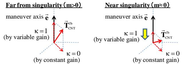
Figure 4 Torque command regulation by CMG gain  $m$
