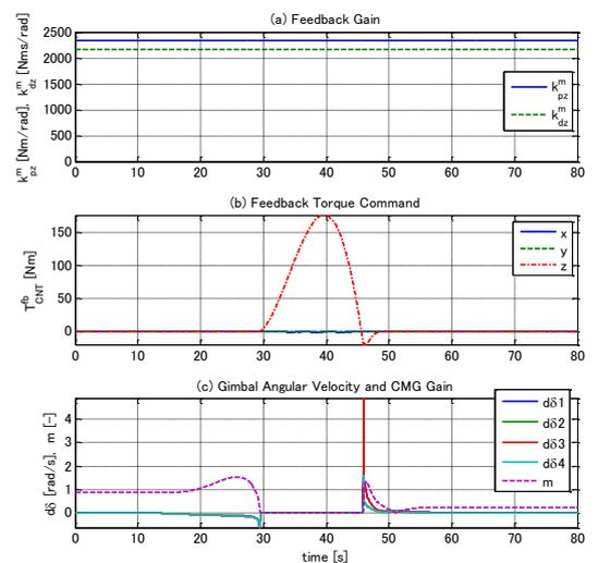
Figure 6 Conventional constant gain feedback control
