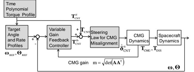
Figure 2 Block diagram of the control and steering laws
