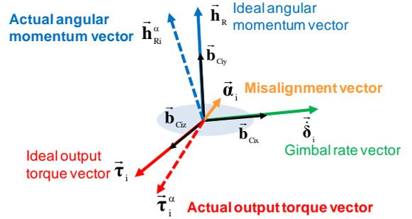
Figure 5 Modeling of the CMG misalignment
