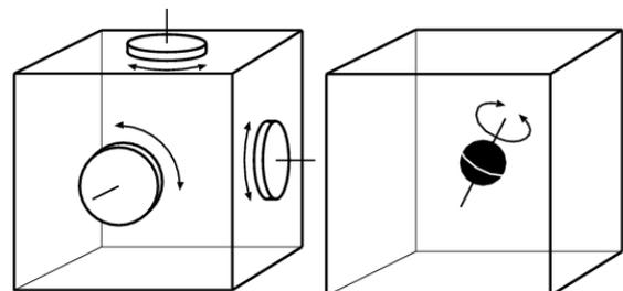
Fig.1 Three Dimensional Reaction Wheel
