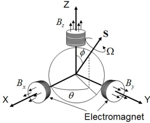
Fig. 2 Formation of electro magnets
