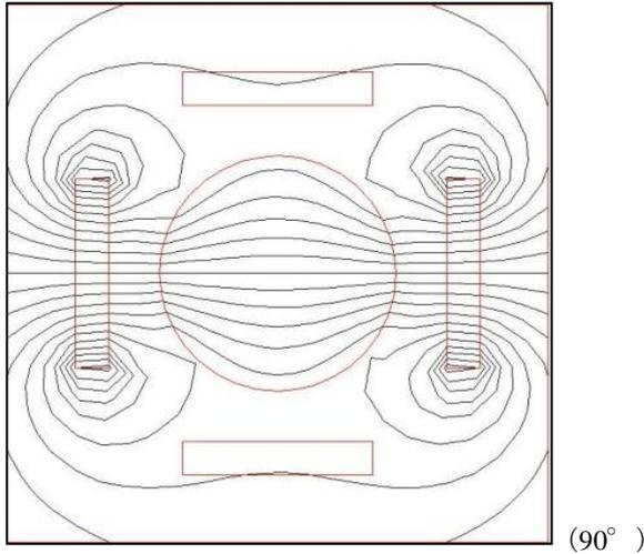
Fig.6 Magnetic flux distribution in cylinder
