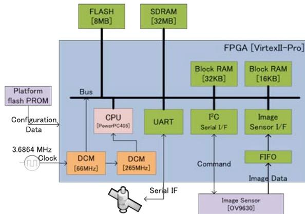
Fig. 4: Block Diagram of HP-IMAP
