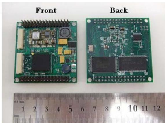
Fig. 3: The processor board microprocessor unit,
