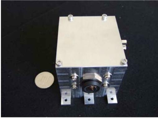
Fig. 1: High-Performance Image Acquisition and Processing unit (HP-IMAP)
