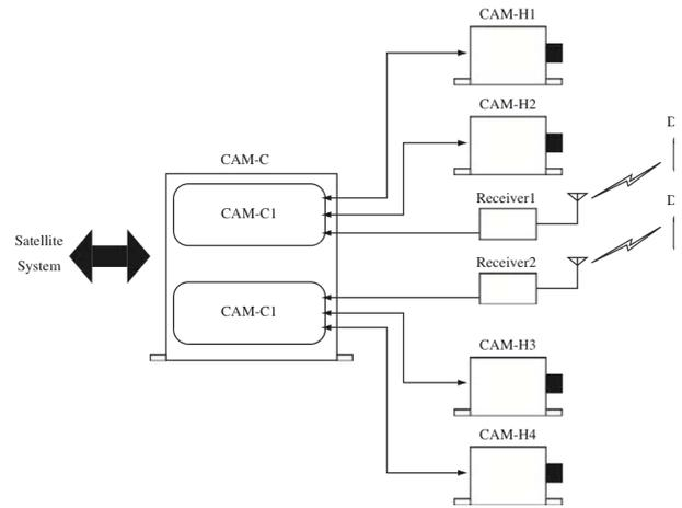
Fig. 2: System Structure of HP-IMAP for IKAROS
