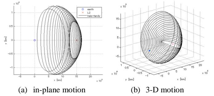
Fig. 2: Halo-Family around L2 in Earth Fixed Coordinate
