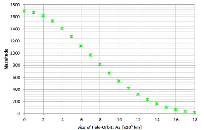
Fig. 3: Variation of the Diverging Magnitude vs Orbit Size
