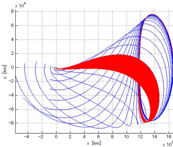
**Fig. 7: Stable Manifolds Designed by Scaling Method**
