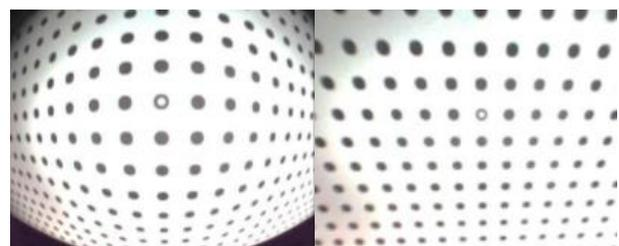
Fig.3 Captured images of the calibration board (left), corrected result (right)
