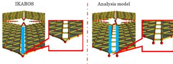
Fig.9 Tip mass arrangement
