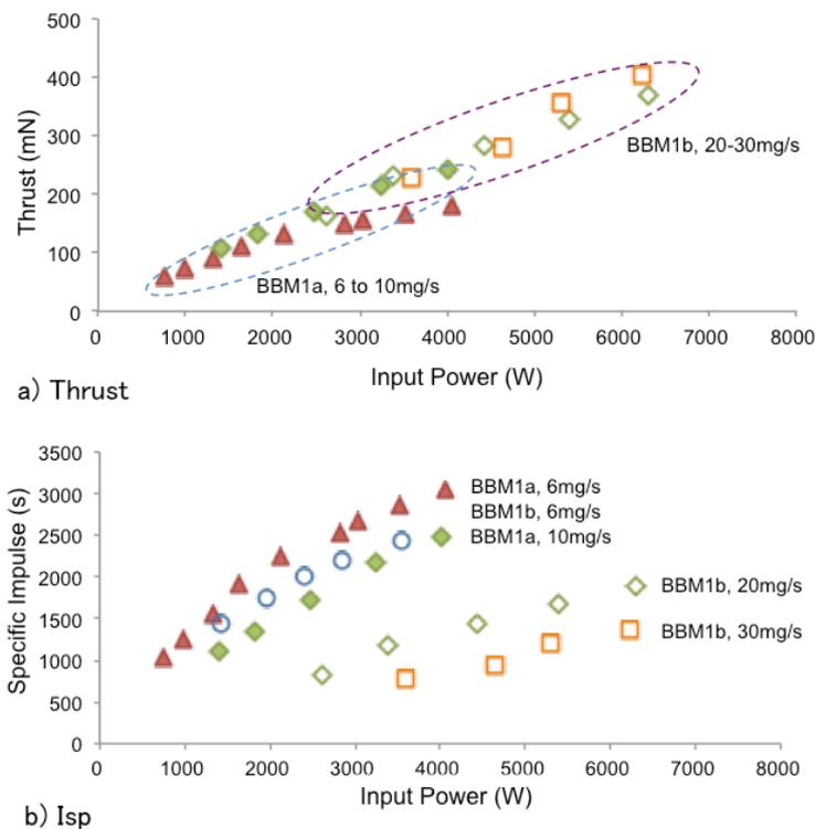
Fig.3 Thrust and Isp characteristics of breadboard models (BBM1).
