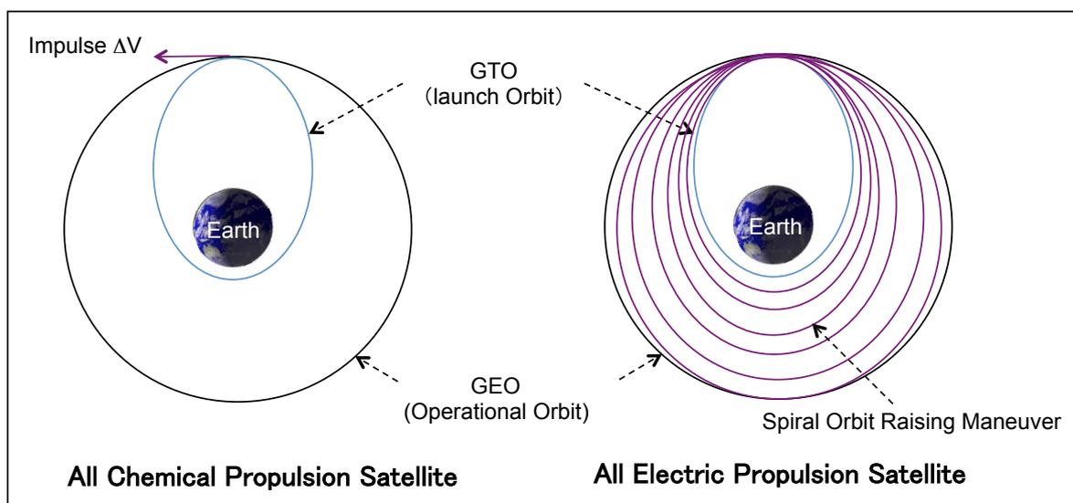
Fig.1 Application of all electric propulsion system to geostationary satellite: all electric propulsion satellite features high payload ratio against ordinary all-chemical propulsion satellite because most delta-V necessary for GTO to GEO transfer is provided via high-Isp electric propulsion.
