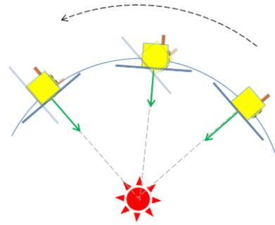
Figure 1. Image of Sun-tracking motion
