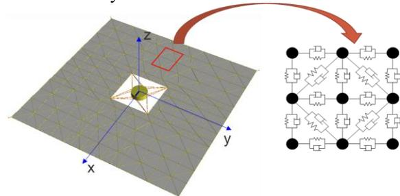
**Fig.5 Concept of Multi Particle Method**
