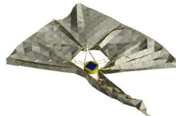
**Fig.11 Asymmetric deployment of Improved MPM**
