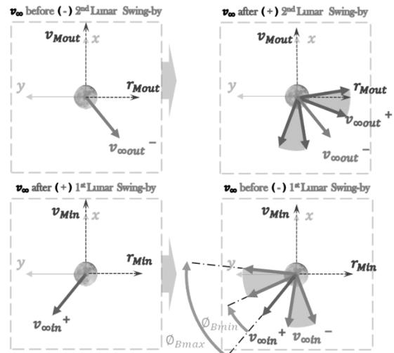
Fig.5 Geometry of Sequential Lunar Swing-by
