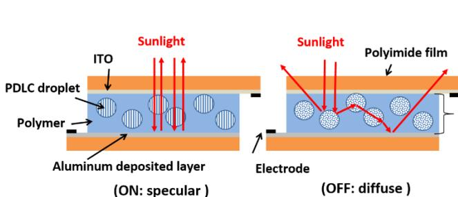
Fig. 1 Mechanism of the RCD.
