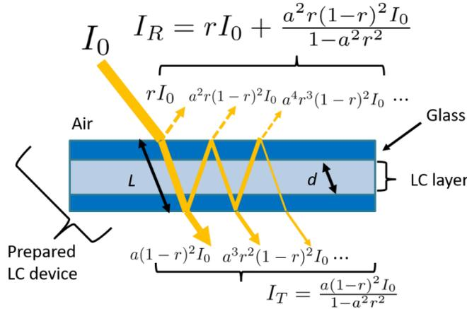
Fig. 4 Transmitted and reflected light.
