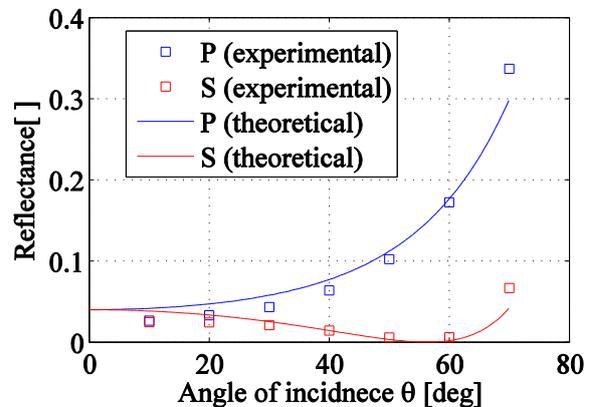
Fig. 7 Reflectance at the interface between the glass and air.
