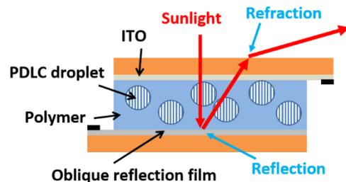
Fig. 2 Concept of the A-RCD.
