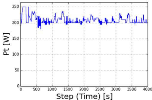
Fig. 12. The total power consumption with the autonomous dispersed control and the temperature limits
