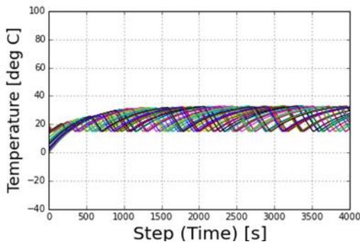
Fig. 11. The temperature of all the channels with the autonomous dispersed control and the temperature limits
