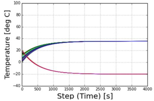
Fig. 8. The temperature of all the channels with the autonomous dispersed control
