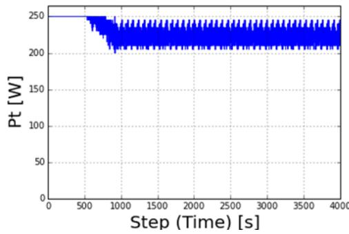
Fig. 7. The total power consumption without the autonomous dispersed control
