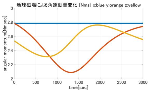
Fig.7 History of angular momentum which is calculated from the residual magnetic torque (Analyzed data) (Blue: X axis, Orange: Y axis, Yellow: Z axis)
