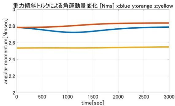
Fig.6 History of angular momentum which is calculated from the gravity-gradient torque (Analyzed data) (Blue: X axis, Orange: Y axis, Yellow: Z axis)
