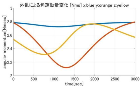
Fig.8 History of angular momentum which is calculated from the total disturbance torque (Analyzed data) (Blue: X axis, Orange: Y axis, Yellow: Z axis)
