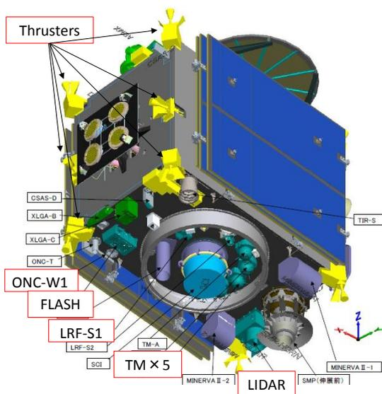
Fig.2 Sensors and actuators mounted positions
