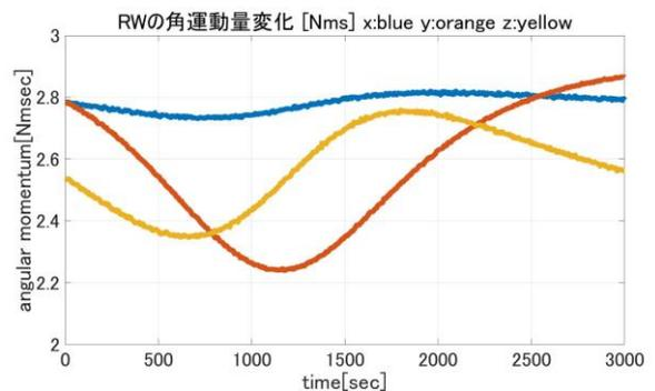
Fig.4 History of RW angular momentum (Telemetry data) (Blue: X axis, Orange: Y axis, Yellow: Z axis)
