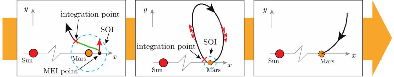
Fig. 4 Conceptual diagram of patched three-and-two-body method using the Sphere of Influence of Mars. Green line is the coasting phase in three-body problem. Black line represents the thrust phase is two-body problem. The three-body and two-body trajectories are integrated at the edge of the Sphere of Influence. Red arrows represent thrust.
