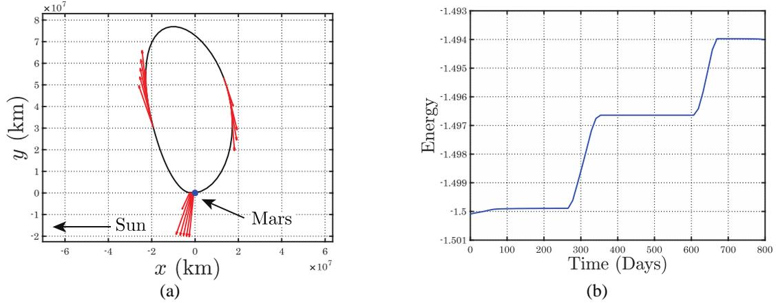
Fig. 6 (a) Optimized two-body trajectory in TOF of 1.2 Martian year,  $\Delta V_{MEI} = 867.3$  m/s, transition from the three-body system to the two-body system at the edge of sphere of influence. (b) The relation of time and expected three-body energy calculated along the trajectory.
