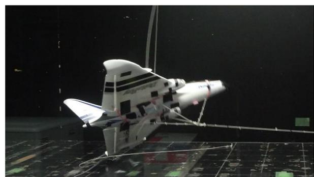
Fig.9 Wind tunnel test of a tethered aircraft (HSWGJapan)
