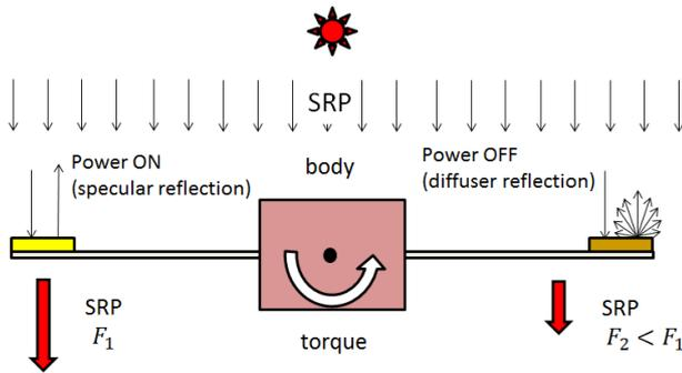
Fig. 1.2. Controlling attitude of IKAROS by RCD.
