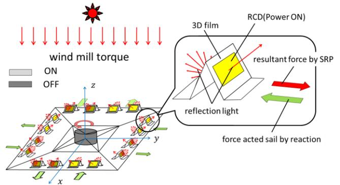
Fig. 1.4. Loading on RCD in three dimensional.
