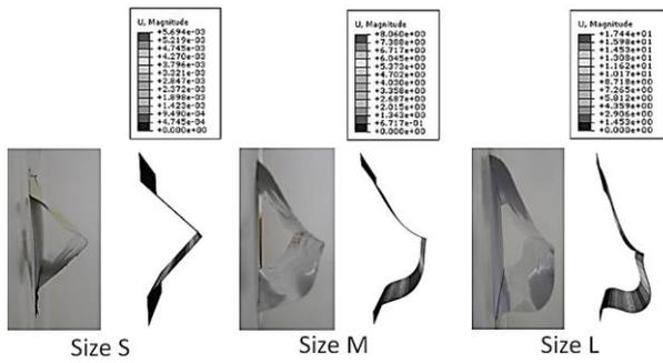
Fig. 2.2. Comparison result of extension experiment and FEM analysis.
