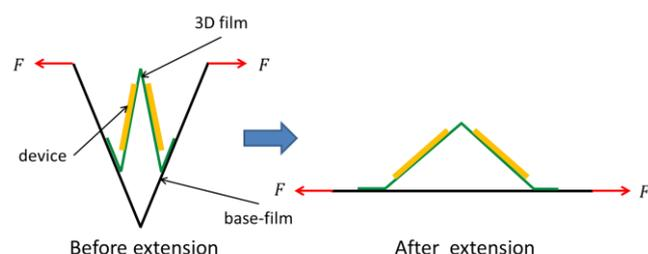
Fig. 1.1. Design of loading three-dimensional thin-film structure.
