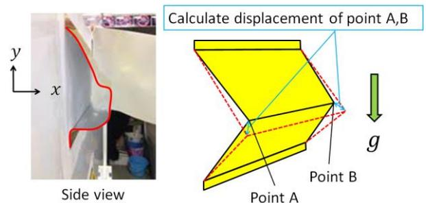
Fig. 2.1. Gravity environment experiment FEM analysis model.
