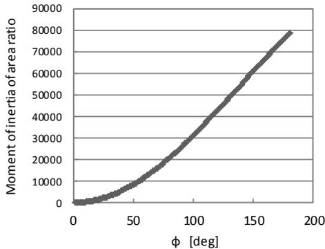
Fig. 6 The moment of inertia of area of comparison between a flat and arc
