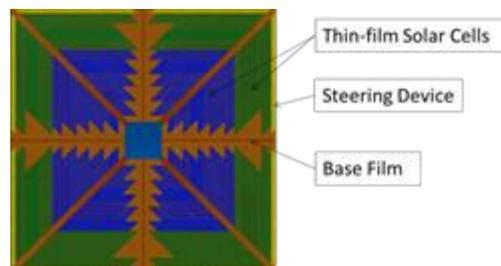
Fig. 3 Next Solar Power Sail Membrane Surface
