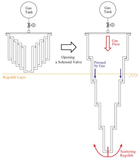
Fig. 1 Concept of Excavation
