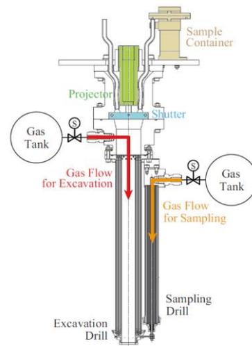
Fig. 2 Concept of Subsurface Sampling Device
