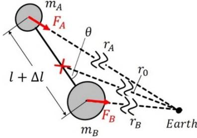
Fig.7 Forces acted on satellite due to the Earth's gravitational force
