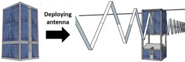
Fig.1 Antenna deployment process of cubesat
