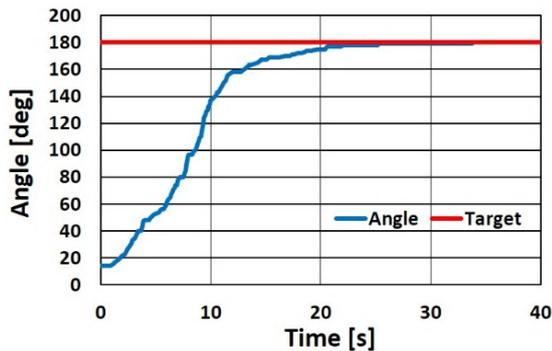
Fig.5 Experimental result of antenna rotation angle
