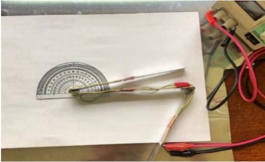
Fig.4 Experimental set-up of antenna deployment
