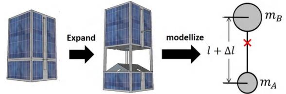
Fig.6 Modeling of satellite of body eccentric model
