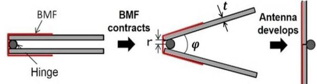
Fig.3 Antenna deployment mechanism
